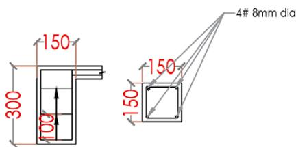
**Figure 3.** Section and plan of the column with reinforcement details.
