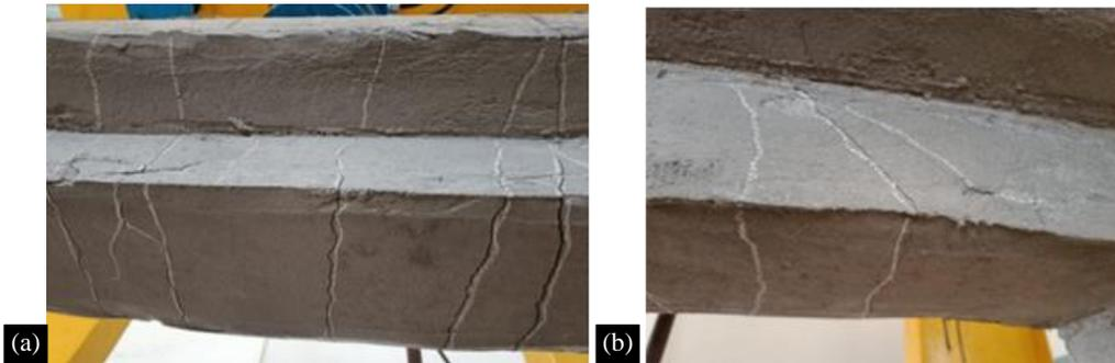
**Figure 13.** Close-up view of flexure and shear cracks in specimen FRCM-1LF.
