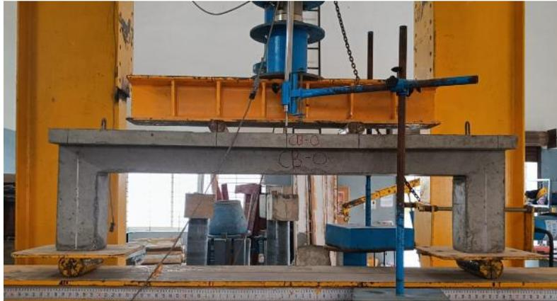
**Figure 11.** Set-up of control beam specimen (CB-0).
