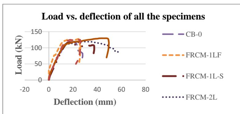
**Figure 16.** Load vs. deflection of all the specimens.
