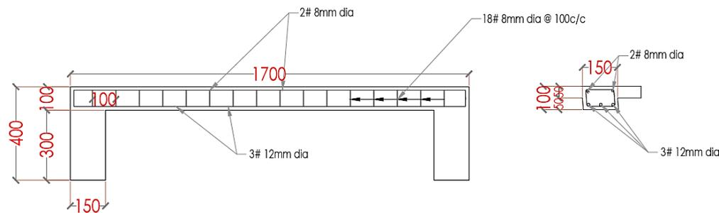
**Figure 2.** Longitudinal-section and cross-section of the beam with reinforcement details.
