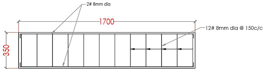
**Figure 1.** Plan of the slab with reinforcement details.
