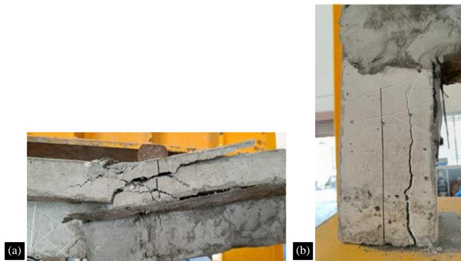
**Figure 15.** Debonding of the slab and column element in specimen FRCM-2L.
