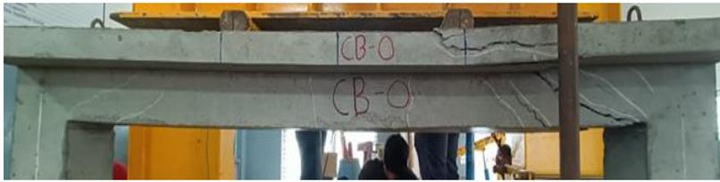
**Figure 12.** Close-up view of shear cracks in specimen CB-0.
