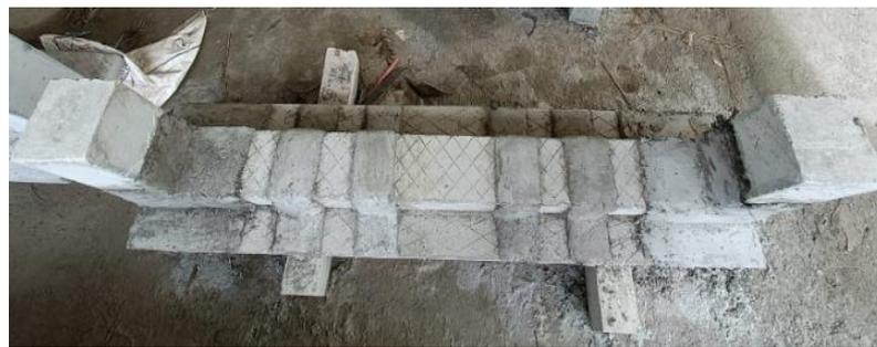
**Figure 8.** Application of FRCM in one layer-strip form.
