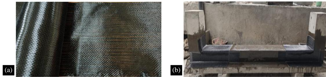
**Figure 10.** (a) CFRP wrap and (b) Beam wrapped with CFRP.
