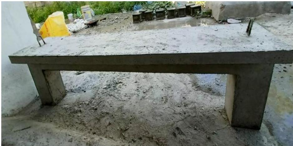
**Figure 4.** T-Beam and C-frame specimen.
