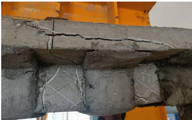
**Figure 14.** Shear cracks in specimen FRCM-1L-S.
