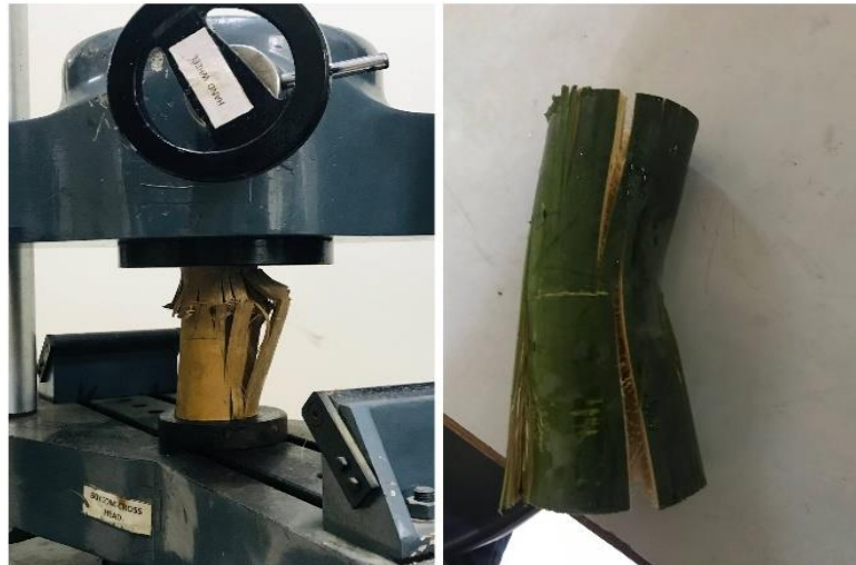
Fig 7 (Failure of bamboo)
