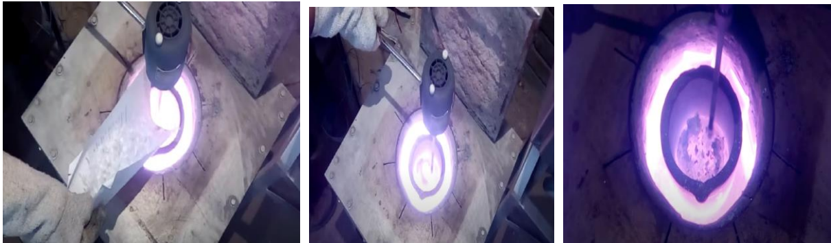
Figure 1. Experimental setup of stir casting Process
