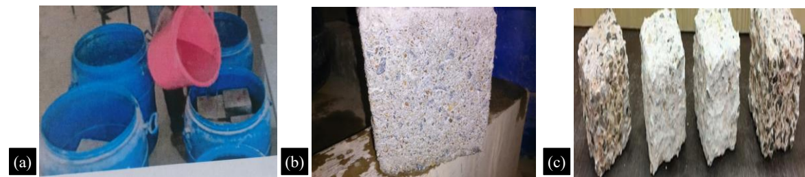
Figure 3. (a-c) Testing and tested samples after immersion for 90 days–sulphate attack.
