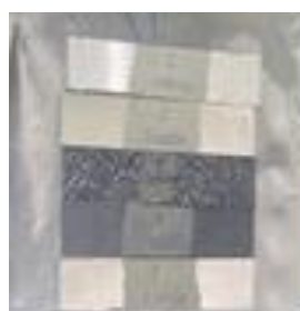
Figure 3. Specimens for corrosion test.
