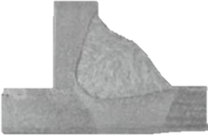
Figure 9. CMT dynamic working on steel with ER70S-6 filler wire.
