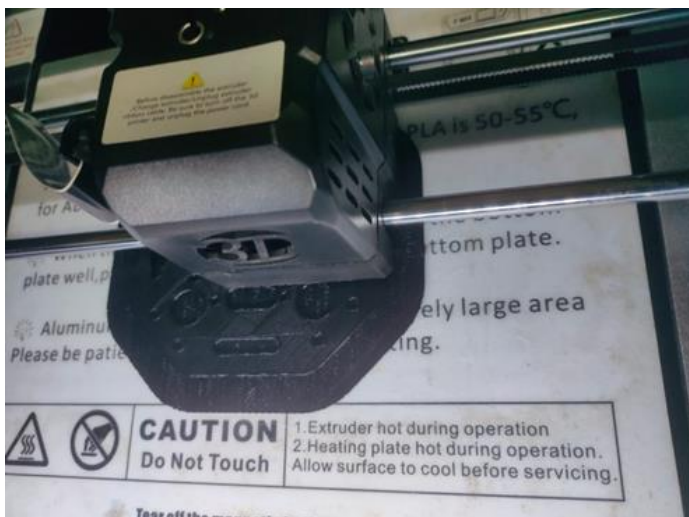
Figure 10. 3D printing of Frame.
