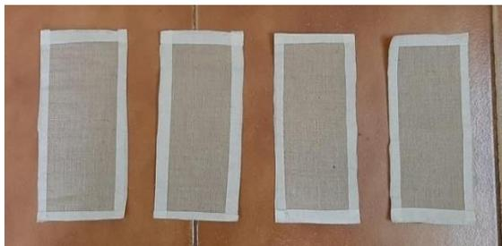
(a). Preparation of flax fibre and sealing the edges of fibre
