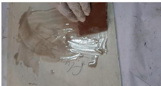
(c). Applying first layer epoxy mixture on steel plate
