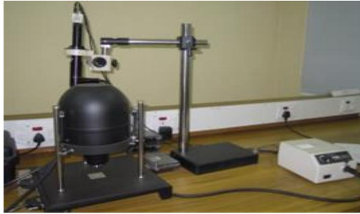
**Fig. 2:** AFM (Model: NT-MDT) Solver-4 Used in Surface Roughness Measurement.
