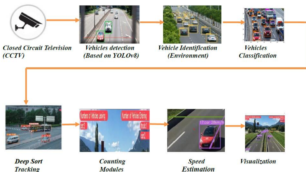
Figure 1. Block diagram of vehicle detection and counting.
