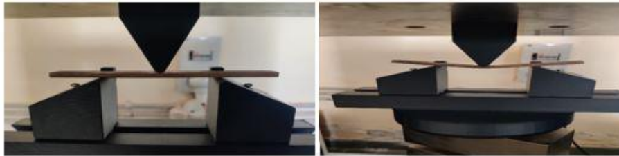
Figure 4. Flexural specimen before failure and after failure.
