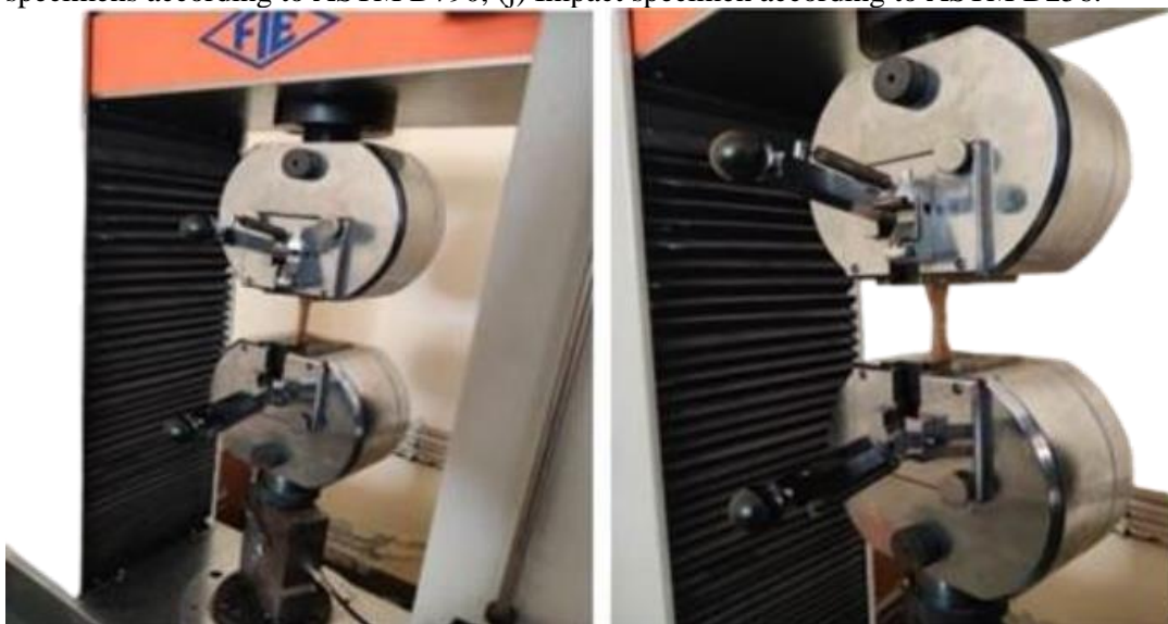
Figure 3. Tensile specimen before failure and after failure.
