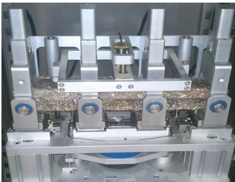
Figure 2. Four-point flexural bending test setup.
