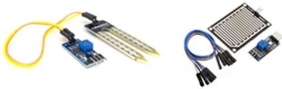
Fig. 4. Soil moisture sensor (left) and rain detection sensor (right).
