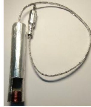
Fig. 4. Probe of EC non-destructive testing device
