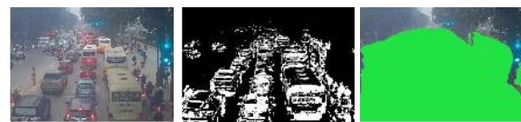
Fig. 5. A video frame of a vehicle flow captured by the camera: a) Original frame; b) Its binarization; c) The area A_{occupied} in the frame marked by green area.
