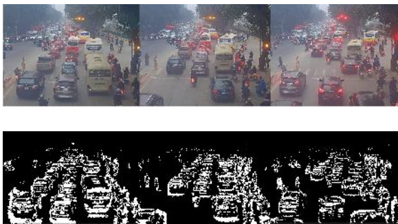
Fig. 7. An example of 3 frames captured phase A-B from the surveillance video sequence and their corresponding binarized images.
