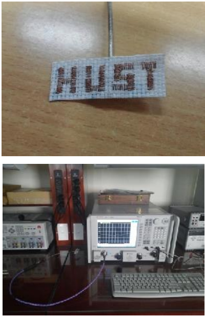
Fig.12. Fabricated antenna and the setup of measurement
