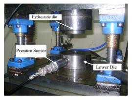
Fig. 10. Overall single sheet metal hydrostatic die
