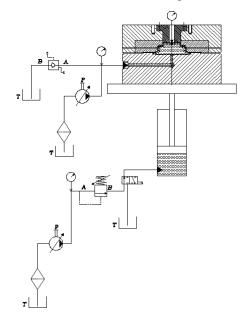
Fig. 9. Hydraulic control system diagram for experiment
