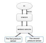
Fig. 6. The diagram of control circuit principle
