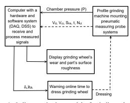
**Fig. 4.** Online-monitoring model of grinding wheel's wear and part's surface roughness for profile grinding ball bearing's inner ring grove [9, 10]
