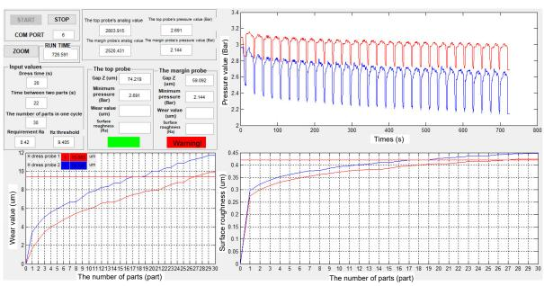
Fig. 10. Software interface after finished grinding 30 parts in one cycle for both the top probe and the margin probe
