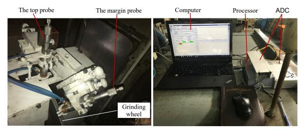
**Fig. 9.** Experimental system measuring grinding wheel's wear for profile grinding ball bearing's inner ring grove after mounting two probes onto profile grinding machine 3MK136B [2, 3]
