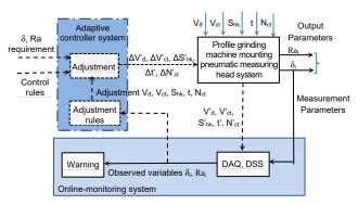
**Fig. 3**. The functional diagram of system to monitor online grinding wheel's wear and part's surface roughness for profile grinding ball bearing's inner ring grove [9, 10]
