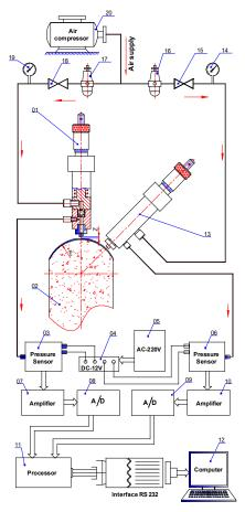
**Fig. 5.** The system diagram for online monitoring grinding wheel's wear in profile grinding process [1-5]
