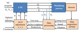
**Fig. 2**. The general structure of an adaptive control system [9, 10]
