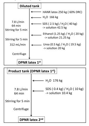
Fig. 1. Operation of Test plant
