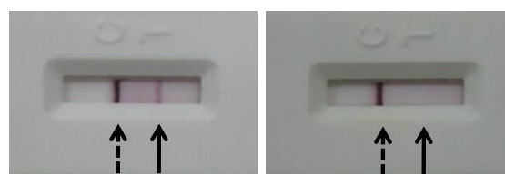
Fig. 11. Generation of complete lateral flow immunoassay test strip. Dashed arrow indicates the control line (C-line), line arrow indicates the test line (T-line)
