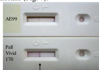
Fig. 7. Different types of the membrane for lateral flow test strip. Signal band is indicated by arrow.
