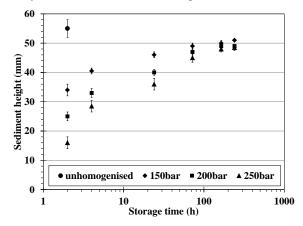
**Fig. 1**. Sediment height of maize suspension as a function of storage time
