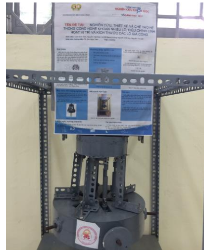
Fig. 10. Overall view of multi-spindle drill head
