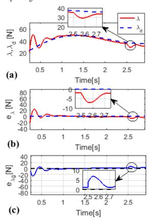
**Fig. 4.** Responding with the change of parameters at t = 2.5[s]: (a) responding force, (b) force tracking error, (c) estimation force error
