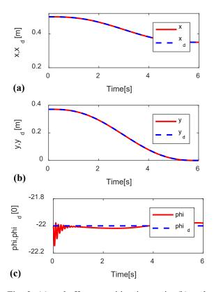
Fig. 2. (a) end-effector position in x-axis, (b) endeffector position in y-axis, (c) orientation of  $\phi$
