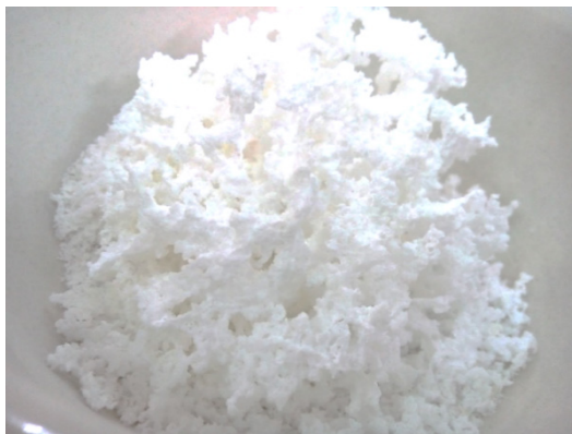
Fig.2 Photograph of combustion-synthesized MgAl_2O_4 product
