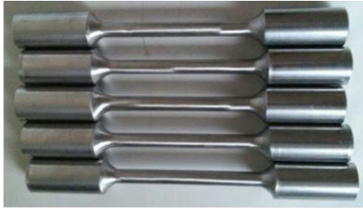
Fig. 1. Rounded specimens for tensile test
