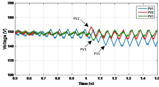
Fig. 7. Voltage reference after tracking on each H-bridge
