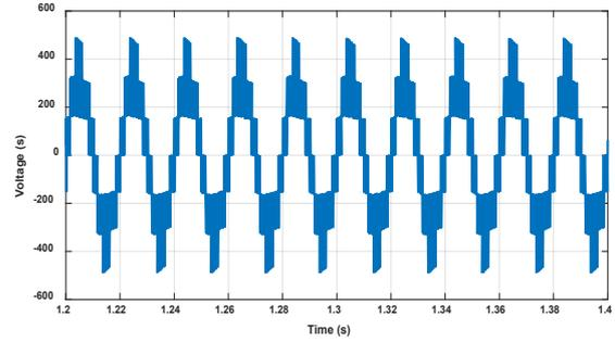
**Fig. 3.** Inverter voltage output
