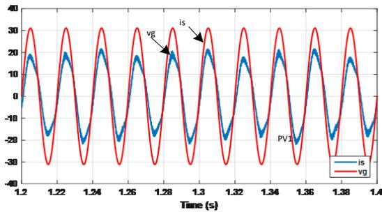
Fig. 8. Output current (10A/div) and grid voltage waveforms (100V/div)
