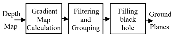
Fig. 4. Block diagram of the ground extraction method based on gradient depth map
