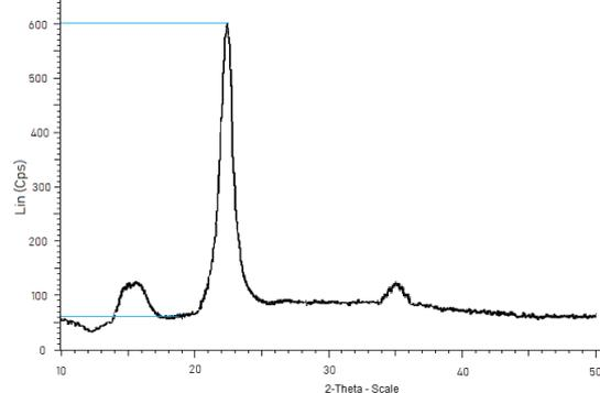
**Fig. 6.** X-ray diffraction patterns of nanocellulose
