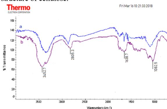
**Fig. 4.** FTIR spectra of (a) bleached *Wood pulp* and (b) nanocellulose.
