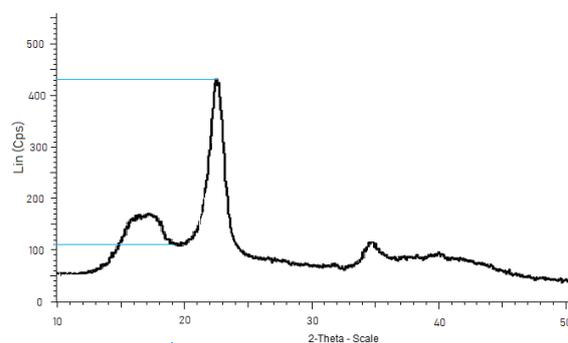
**Fig. 5.** X-ray diffraction patterns of bleached *Wood pulp*
