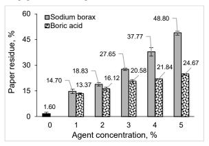
**Fig. 1**. Influence of borax and boric acid concentration on flammability of paper when used separately; impregnation and burning time were 5 min and 30 s, respectively
