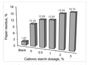
**Fig. 4**. Influence of cationic starch dosage on chemical retention and flammability of paper
