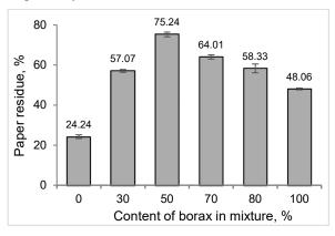
**Fig. 2.** Influence of borax/ boric acid ratio on flammability of paper when used in mixtures; impregnation and burning time were 5 min and 30 s, respectively
