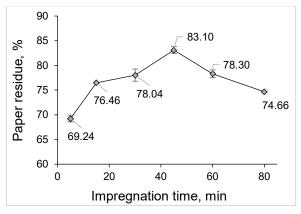
**Fig. 3**. Influence of impregnation time on flammability of paper when using 50/50 ratio of borax/boric acid for impregnation, burning time 30 s
