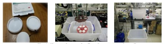
Fig. 1. Chemcatcher sampler, Experiment setup and sampling
