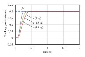
**Fig. 6** Tracking results with different external loads (experiment)
