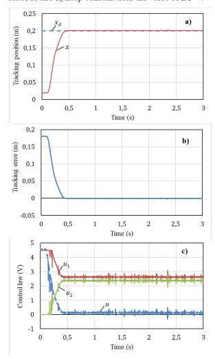
**Fig. 5.** Experimental result: a) tracking position, b) tracking error, c) control law (experiment)
