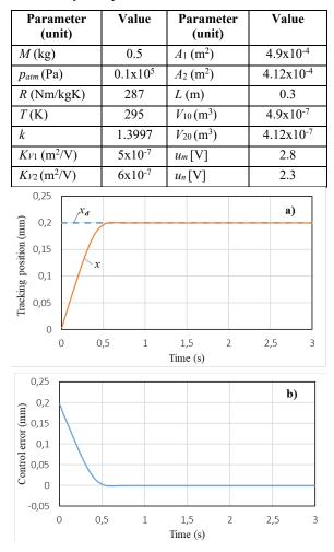
**Fig. 4.** Simulation results: a) tracking position, b) tracking error
