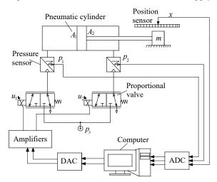
Fig. 1. Schematic of the experimental setup
