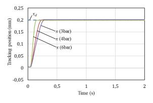
**Fig.** 7 Tracking results with different source pressure (experiment)
