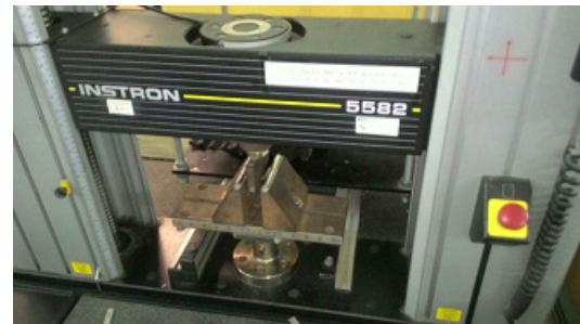
c- Flexural testing
