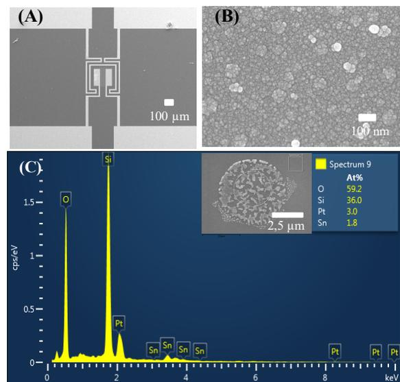
Fig. 2. SEM images of (A) a full chip, (B) SnO<sub>2</sub> thin film on SiO<sub>2</sub> and (C) EDS analysis of SnO<sub>2</sub> thin film sensitized with Pt islands.
