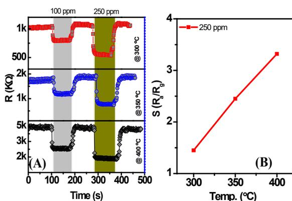
Fig. 3. (A) Transient response of bare  $SnO_2$  and (B) Sensor response as a function of operating temperature.
