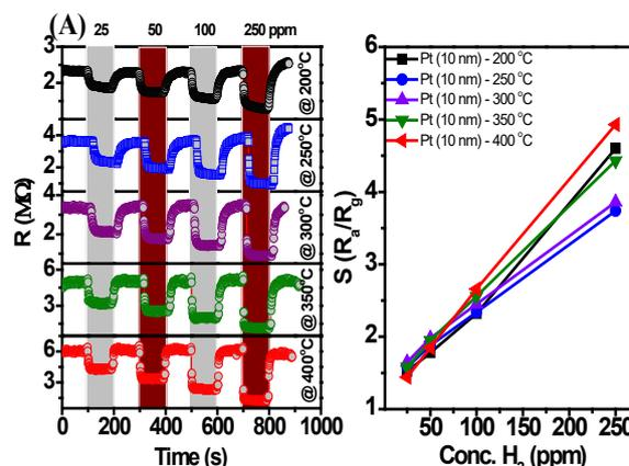
Fig. 4. Transient response of  $SnO_2/Pt$  (10 nm) island sensors (A). Sensors response as a function of gas concentration (B).
