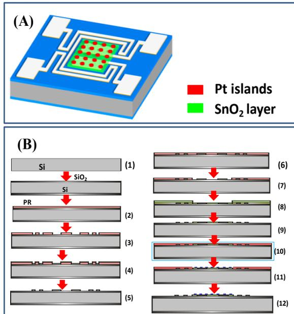
Fig. 1. Design layout (A) and sensor fabrication (B) Ref [14].
