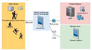
Fig. 2. Architecture of the proposed wireless fall warning system
