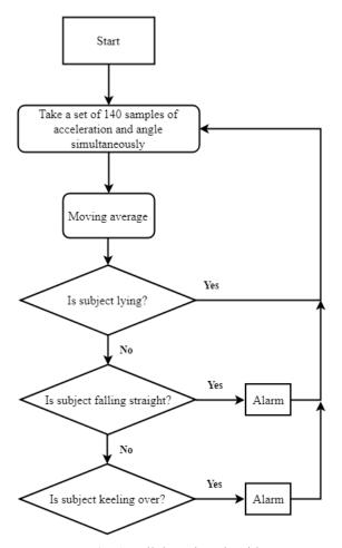
Fig. 1. Fall detection algorithm.
