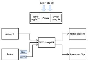
Fig. 3. Block diagram of motion sensor module
