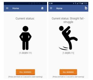
**Fig. 7.** a. Graphical interface of a smartphone shows status of person in Activities of Daily Living; b. Manual warning button and straight fall – struggle symbol when fall is detected.
