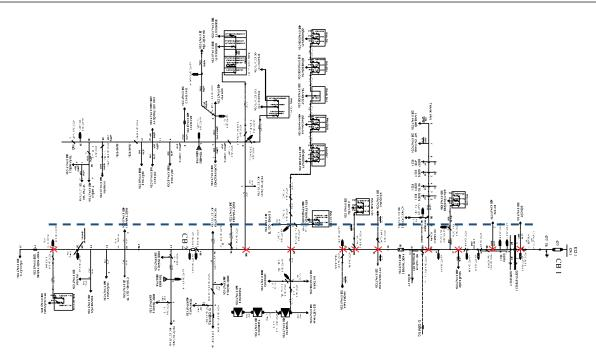
**Fig. 5.** Studied distribution network including main feeder (dash line) and final sectionalizers' placement (red X mark)
