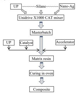
Fig. 1. The diagram of dispersion nano-silver and producing composite
