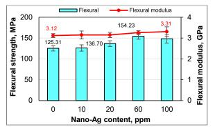
**Fig. 5.** The effect of the nano-silver content on the flexural properties of composite
