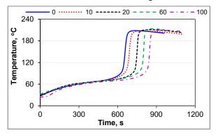
**Fig. 4.** The effect of the nano-silver content on the heat of curing reaction
