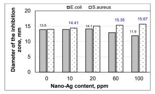
**Fig. 3.** The effect of nano-silver content on the diameter of inhibition zone
