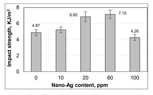
**Fig. 7.** The effect of the nano-silver content on the impact strength of composite
