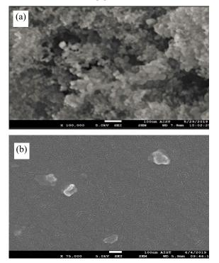
Fig. 8. The field emission scanning electron micrograph of nano-silver (a) and nanocomposite (b)
