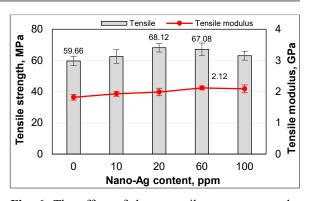
**Fig. 6.** The effect of the nano-silver content on the tensile properties of composite
