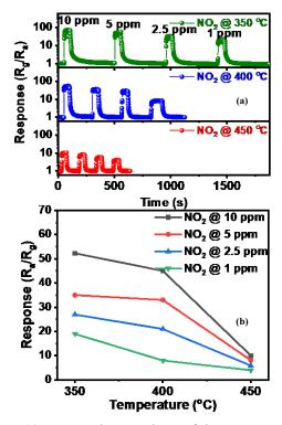
Fig. 5. (a)  $NO_2$  sensing transients of the  $SnO_2$  NFs at various operating temperatures and (b) Gas responses as a function of the  $NO_2$  concentration at different temperatures.
