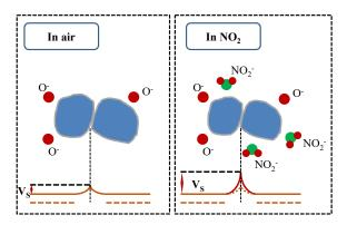
**Fig.7.** Schematic illustration the NO<sub>2</sub> sensing mechanism of the SnO<sub>2</sub> NFs.
