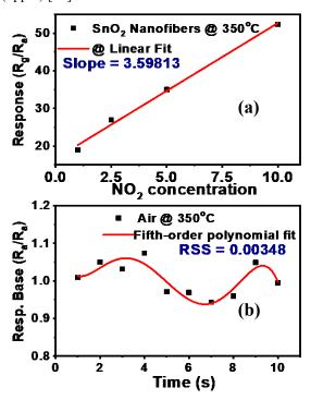
**Fig. 6.** (a) Slope for DL calculation of the SnO<sub>2</sub> NFs sensors. (b) fitted values of residual sum of square (*RSS*).
