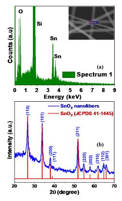
Fig 4. (a) The EDX spectrum and (b) XRD pattern of the  $SnO_2$  NFs.
