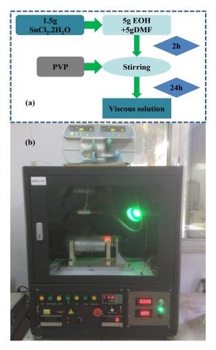
**Fig.2.** (a) The procedure of preparation of the electrospinning solution. (b) real electrospinning system for the NF synthesis
