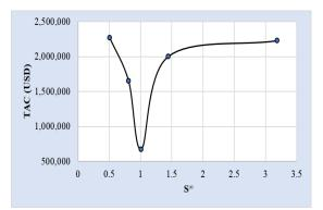
**Fig. 7.** The effect of solvent selectivity on the total annual cost of an enhanced distillation operation for - Ethanol-Water mixture
