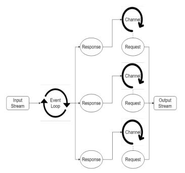
Fig. 5. Application architecture of CoTCP Client
