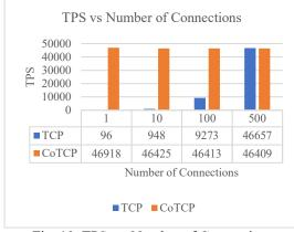
Fig. 10. TPS vs. Number of Connections
