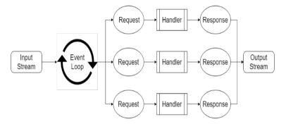
Fig. 6. Application architecture of CoTCP server
