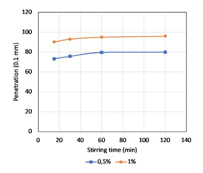
Fig. 8. Effect of stirring times to the needle penetration
