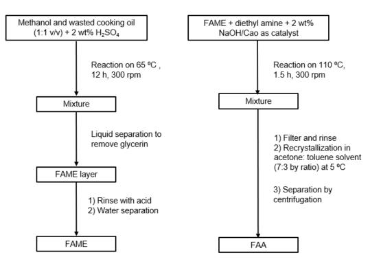
Fig. 1. Synthesis procedure of FAA from waste cooking oil
