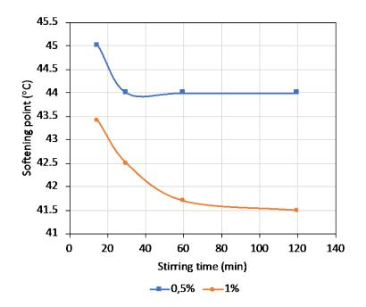
Fig. 7. Effect of stirring times to softening point
