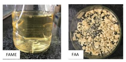
Fig. 2. Image of the synthesized fatty acid methyl ester (FAME) and fatty acid amide (FAA)
