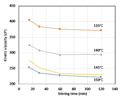
Fig. 6. Effect of temperature to kinetic viscosity at different stirring times
