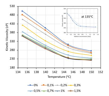
Fig. 5. Effect of temperature to kinetic viscosity at different additive concentrations
