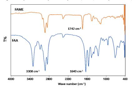
Fig. 3. FTIR spectra of fatty acid amide (FAA) and fatty acid methyl ester (FAME)
