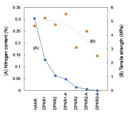
Fig. 9. Relationship between nitrogen content and mechanical properties of natural rubber
