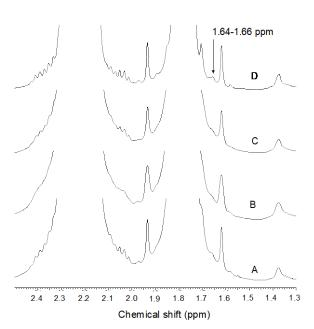
Fig. 6. Signals of phospholipid and phosphate groups of (A) HANR-AE, (B) DPNR1-A-AE, (C) DPNR2-A-AE and (D) DPNR3-A-AE
