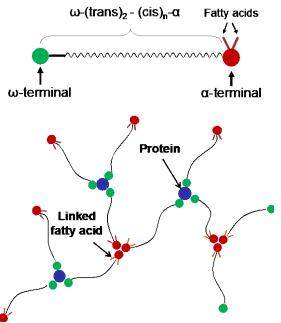
Fig. 1. Fundamental structure of natural rubber and branch points in natural rubber
