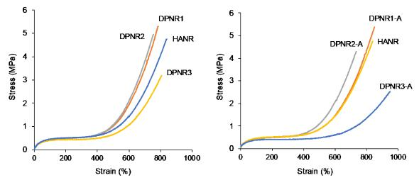
Fig 8. Stress-strain curves of DPNR1, DPNR2, DPNR3 and DPNR1-A, DPNR2-A, DPNR3-A
