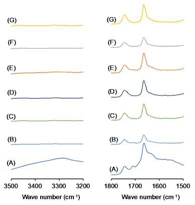
Fig. 3. Fourier transform infrared spectra for (A) HANR, (B) DPNR1 and (C) DPNR2, (D) DPNR3, (E) DPNR1-A, (F) DPNR2-A and (G) DPNR3-A
