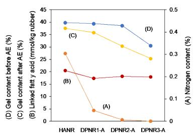
Fig. 4. Relationship between nitrogen content (A), linked fatty acids content (B) and gel content after AE (C), and gel content before AE (D) of HANR, DPNR1-A, DPNR2-A and DPNR3-
