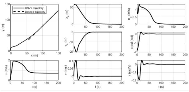
Fig. 4. Trajectory tracking performance - Simulation Run #3
