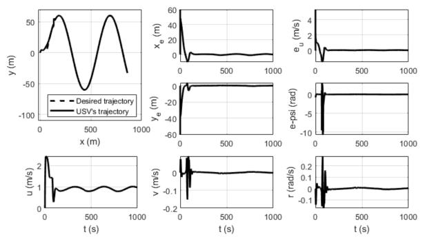
Fig. 9. Trajectory tracking performance - Simulation Run #8
