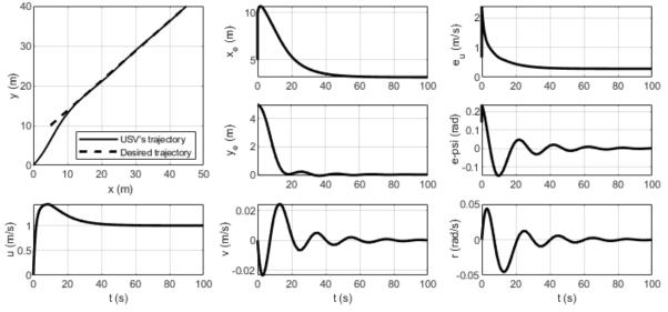
Fig. 2. Trajectory tracking performance - Simulation Run #1
