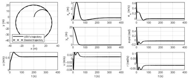
Fig.5. Trajectory tracking performance - Simulation Run #4
