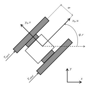
Fig. 1. The USV's configuration and dynamics
