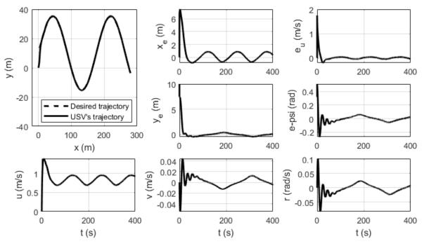
Fig. 10. Trajectory tracking performance - Simulation Run #9
