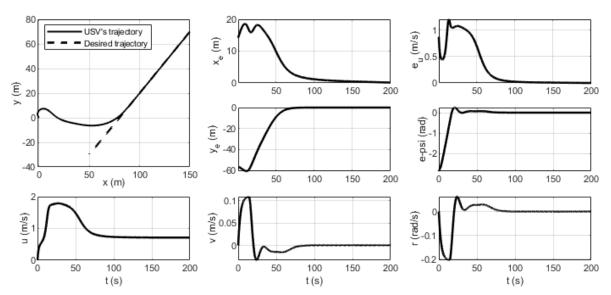
Fig .3. Trajectory tracking performance - Simulation Run #2
