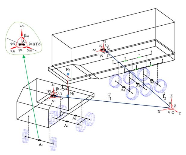
Fig. 2. Tractor semitrailer vehicle coordinate systems
