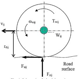
Fig. 4. Schematic of wheel dynamics
