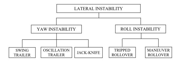
Fig. 1. Lateral instability categorization of tractor semitrailer vehicle
