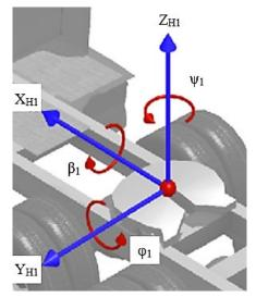
Fig. 5. Model of fifth wheel hitch
