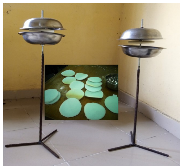
Fig. 1. The locally fabricated PUF passive sampler (inset shows the PUF)
