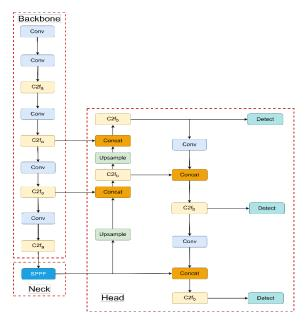
Fig. 6. YOLOv8 architecture.
