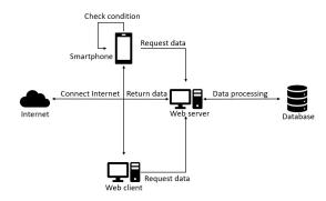
Fig. 3. Logic model to implement the system
