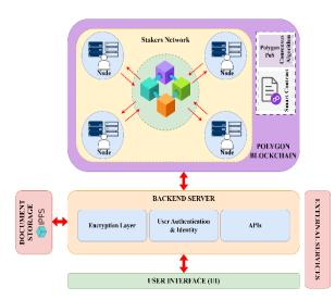
Fig. 5. Basic architecture of Blockchain-based Document Management.
