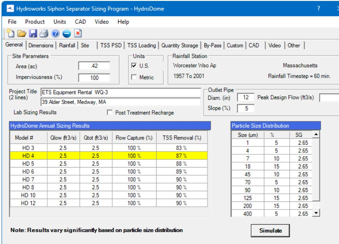
Figure 11. ETS Equipment Rental Separator Sizing Results – WQ-3
