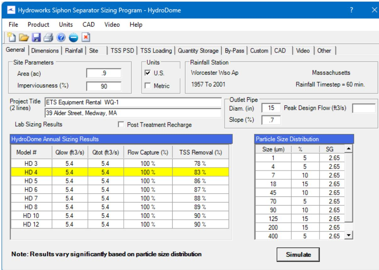
Figure 9. ETS Equipment Rental Separator Sizing Results – WQ-1
