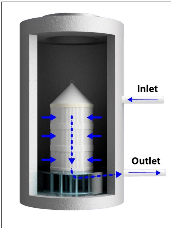
**Figure 3. Hydroworks HydroFilter Operation**
