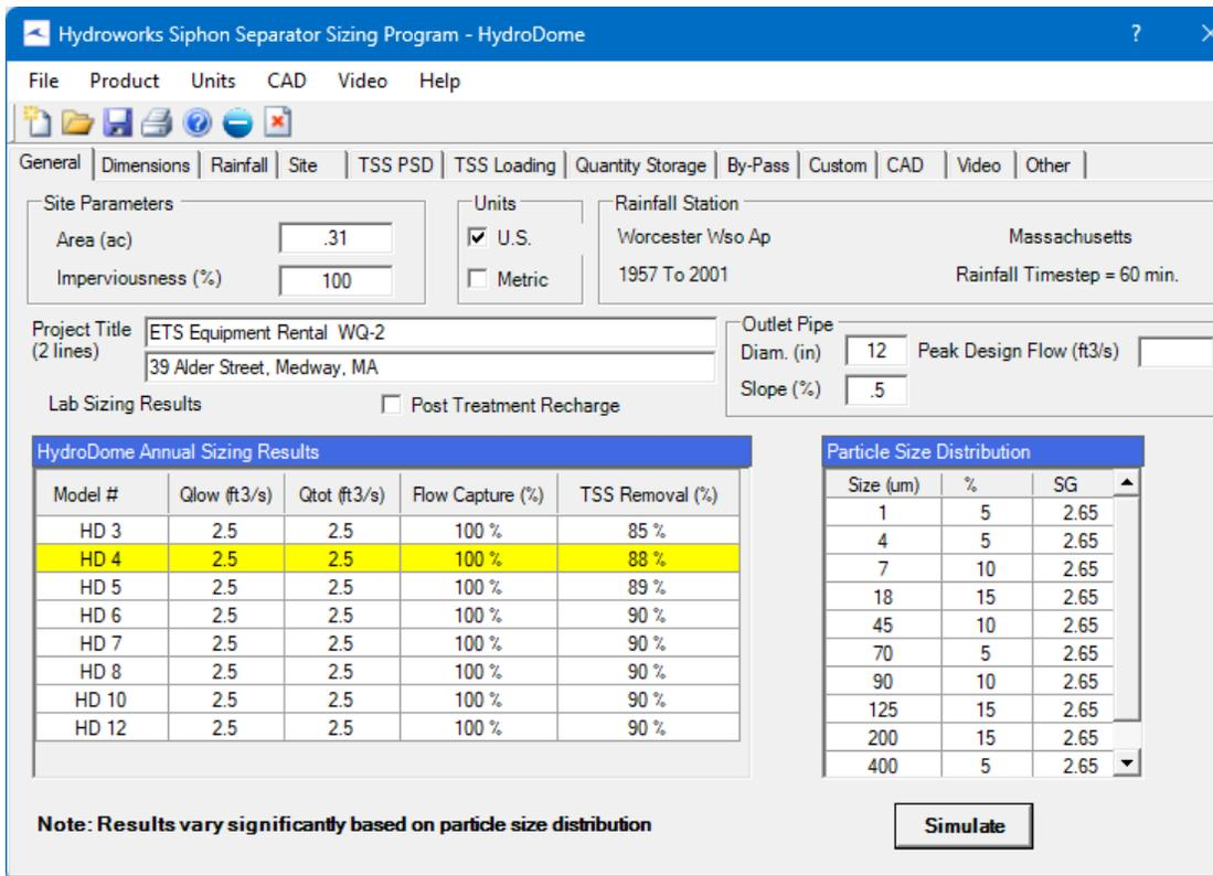
Figure 10. ETS Equipment Rental Separator Sizing Results – WQ-2
