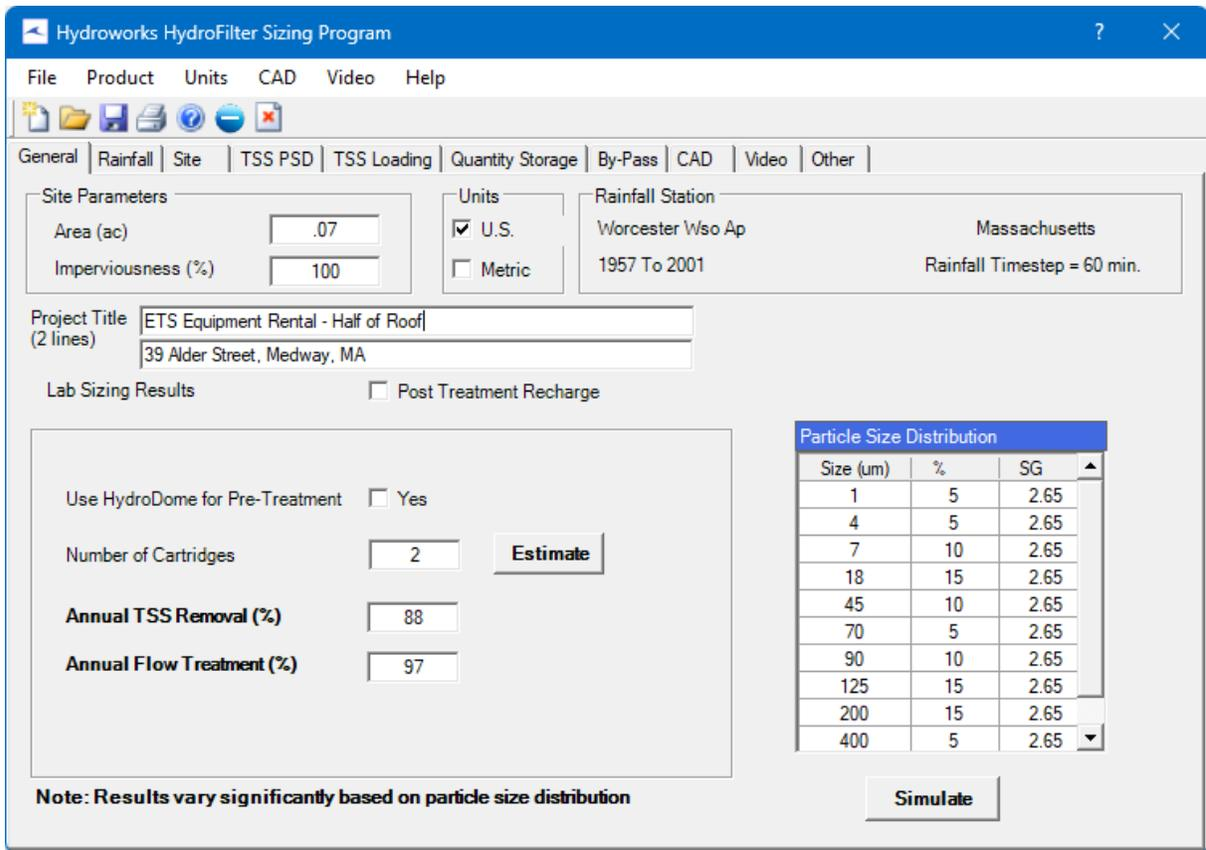
Figure 12. ETS Equipment Rental Separator Sizing Results – HF-1 & HF-2
