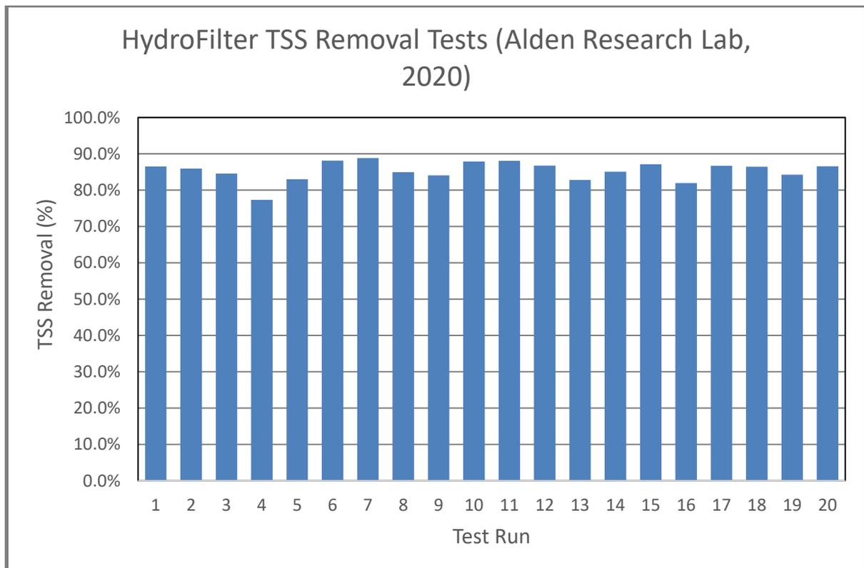
**Figure 8. HydroFilter NJDEP Test Results**
