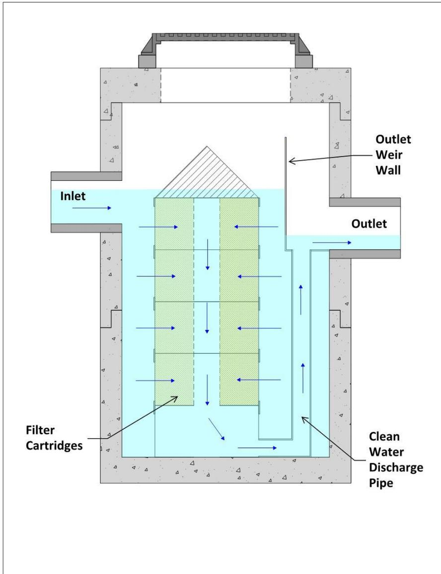
**Figure 1. Hydroworks HydroFilter Operation – Standard Filter**
