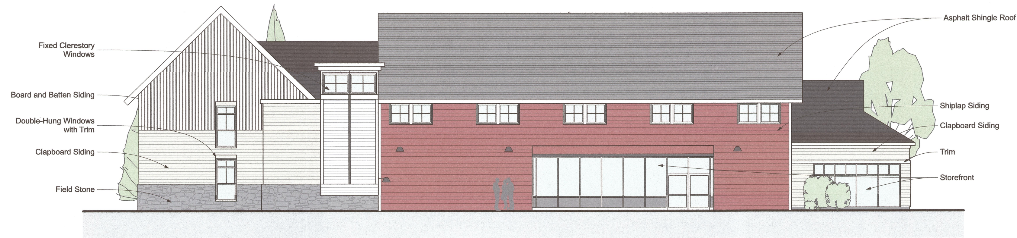
3 NORTH ELEVATION FROM SECURE COURT Scale: 3/32" = 1'-0"
