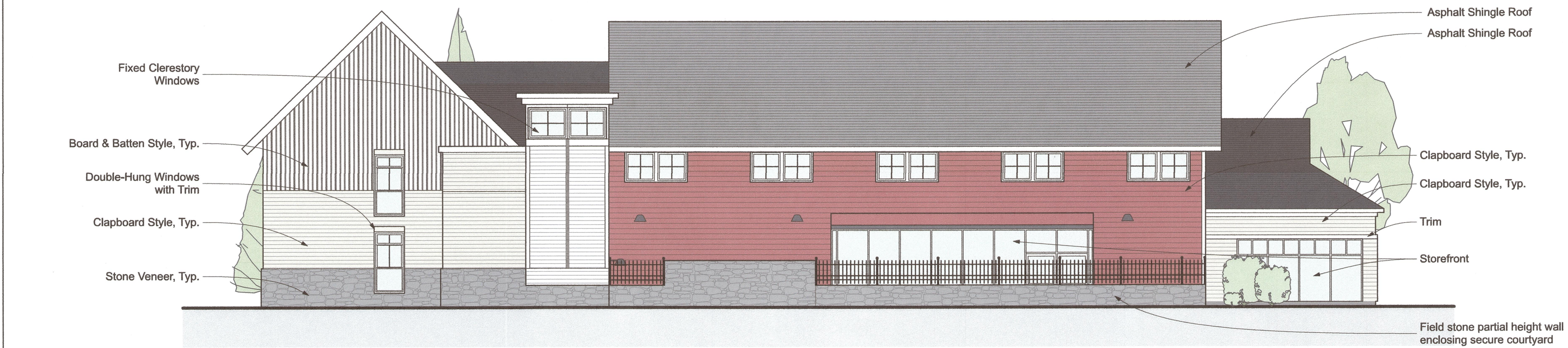
5 NORTH ELEVATION FROM STREET Scale: 3/32" = 1'-0"
