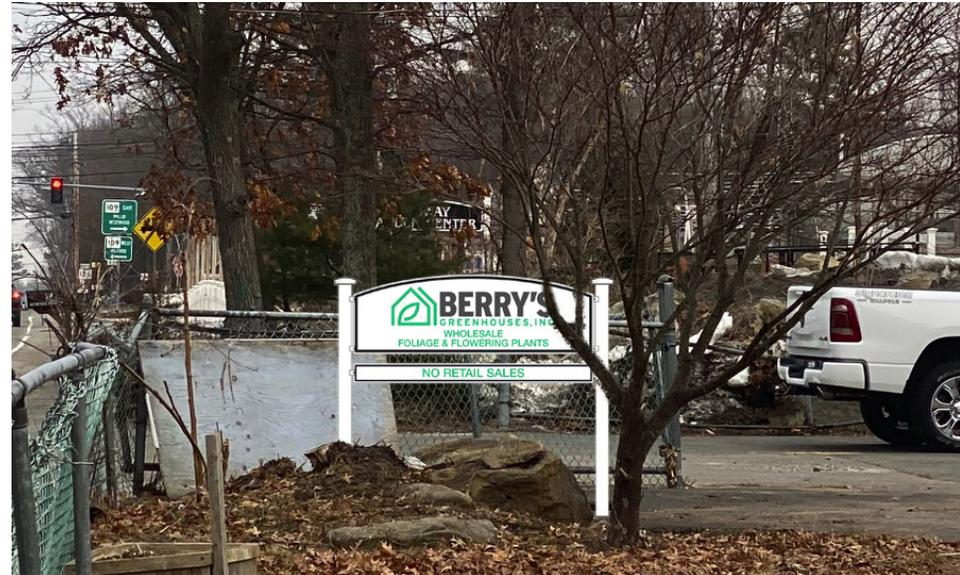
Post and Panel sign with pvc sign panels and high performance vinyl applied to sign faces. Pressure Treated 4x4 posts sleeved with PVC sleeves cemented into the ground.
